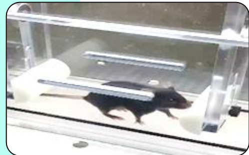
DigiGait™ with a mouse in the running chamber conducting gait analysis.
